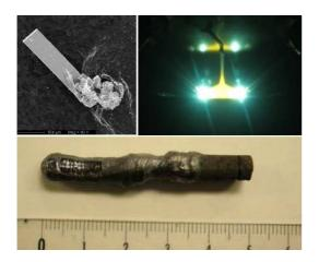
Fig. 1:PrOs<sub>4</sub>Sb<sub>12</sub> single crystal grown out of Sb flux (top left), single crystal growth of UCoGe in the tetra arc furnace (top right)) and  $Sr_{12}Ca_2Cu_{24}O_{41}$  crystal grown by the TSFZ technique (bottom).
