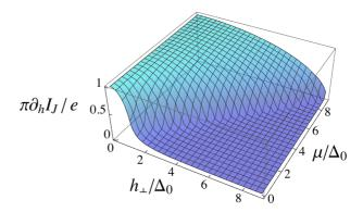
FIG. 3. (Color online) The slope of the anomalous Josephson current in short junctions as a function of the magnetic field  $h_{\perp}$  perpendicular to the spin quantization axis and the chemical potential. The slope remains close to its quantized value as long as  $h_{\perp} \ll \sqrt{\Delta_0^2 + \mu^2}$ .
