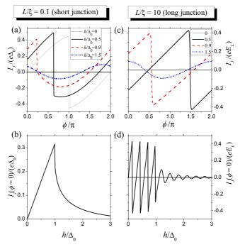
FIG. 1. (Color online) Anomalous Josephson effect in short [ $L=0.1\xi$ , panels (a) and (b)] and long [ $L=10\xi$ , panels (c) and (d)] S-QSHI-S junctions. Panels (a) and (c) show the current-phase relation at temperature  $T/\Delta_0=10^{-3}$  for different values of the applied magnetic field h. Panels (b) and (d) show the anomalous Josephson current at  $\phi=0$  as a function of h.
