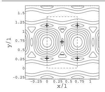
FIG. 3. Square asymmetric vortex lattice described by the Landau level functions n = 2 formed in the presence of orbital and spin effects. The profiles of the amplitude of the superconducting order parameter are shown. The dashed line represents the unit cell with five zeros. Their winding numbers,  $\pm 1$ , are shown. There is one flux quantum per unit cell.
