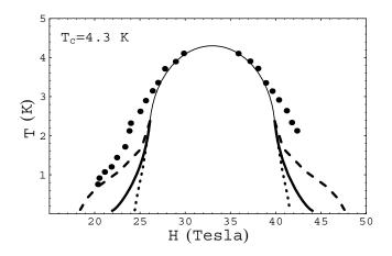
FIG. 1. The dependence of the critical temperature on the magnetic field parallel to the layers in the presence of the Jaccarino-Peter effect. The thin solid curve is the transition from the normal metal to the uniform superconducting state. The dotted (thick) line is the transition to the LOFF state in the isotropic 3D (2D) system, and the dashed line is for the in-plane anisotropic 2D system. Dots are experimental data obtained by resistivity measurements [2].
