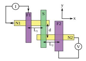
FIG. 1. (Color online) Schematic diagram of the device. The bias current is applied from a ferromagnet  $F_1$  to a normal metal  $N_1$  and nonlocal voltage is measured between  $F_2$  and  $N_2$ .
