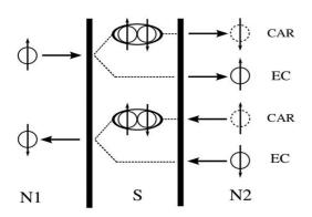
FIG. 2. Nonlocal correlations near the  $N_1SN_2$  structure. Pure spin current is injected from  $N_1$  and a finite spin current is generated in  $N_2$  by CAR and EC. One should note that the direction of the spin currents attributed to CAR and EC are in the same direction and there is no net spin accumulation in the superconductor.
