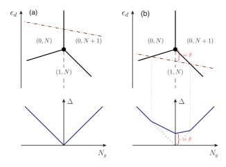
FIG. 5. (Color online) Activation energy  $\Delta$  around a sequential-tunneling peak. (a) Top: fragment of the stability diagram [see Fig. 4(b)] showing the working line (dash-dotted line) outside the anomaly region. Bottom: the  $\Delta$  vs  $N_g$  dependence, corresponding to the top panel. (b) Same as in (a) but with the working line in the anomaly region. The smallest value of  $\Delta$  is  $\delta$ .
