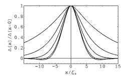
FIG. 2. Self-consistent gap just below the second-order transition line  $h_{cw}(T)$  into a localized domain wall superconducting state at different temperatures  $T = (0, 0.2, 0.4, 0.6, 0.8)T_{c0}$  (from narrowest to widest).
