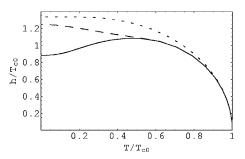
FIG. 1. Phase diagram. The straight line is the critical line  $h_c^{(2)}(T)$  of the second-order transition into a uniform superconducting state. At  $T < T^* = 0.56T_{c0}$ , the transition into a uniform state at  $h_c(T)$  is of the first order (dashed line). The critical line  $h_{cw}(T)$  corresponding to domain wall superconductivity is of the second order (dotted line).
