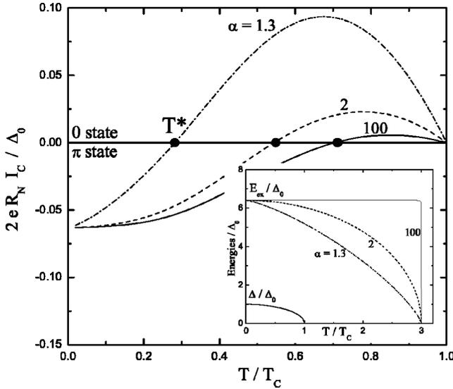
FIG. 7. Crossover in temperature with the additional contribution of a temperature-dependent exchange energy  $E_{ex}(T)$  in a short S/F/S junction with  $E_{Th} = \Delta_0$ ,  $E_{ex}(0) = 6.4 \Delta_0$ , and  $T_{Curie} = 3 T_c$ . Three different dependencies are compared:  $\alpha = 100$ , 2, and 1.3, corresponding to the increasing temperature variations shown in the inset.
