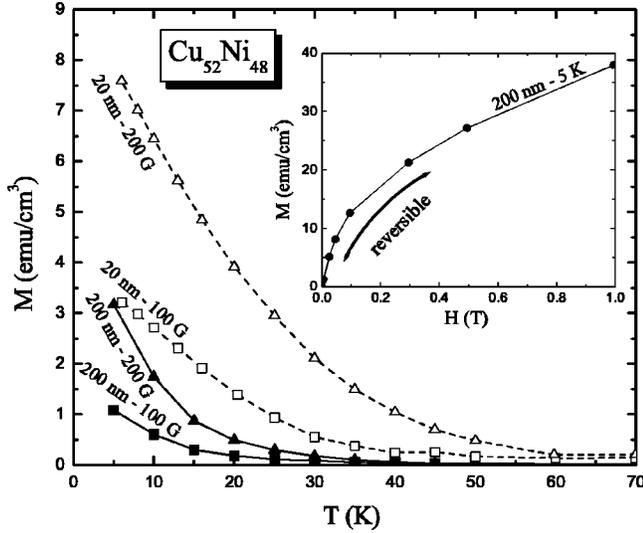
FIG. 9. Magnetization versus temperature for a 20-nm  $\text{Cu}_{52}\text{Ni}_{48}$  layer in a Nb/CuNi/Nb trilayer and for a 200-nm  $\text{Cu}_{52}\text{Ni}_{48}$  single layer. A magnetic field of 100 and 200 G is applied because the remanent magnetization is zero. Inset: reversible magnetization versus magnetic field at 5 K for the 200-nm  $\text{Cu}_{52}\text{Ni}_{48}$  single layer.
