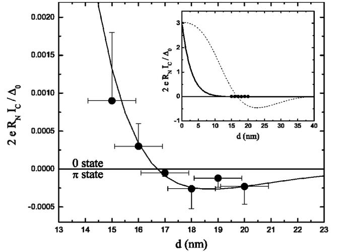
FIG. 14. Critical current of Nb/Cu<sub>52</sub>Ni<sub>48</sub>/Nb junctions at zero temperature versus CuNi thickness compared to the theoretical model with  $E_{ex}(0) = 7.2$  meV and a spin-flip length  $L_{sf} = 2.7$  nm (solid line). Inset: same graph on a larger scale, plus the theoretical curve without spin-flip scattering (dashed line).
