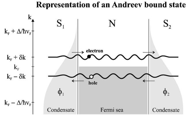
FIG. 1. Electron and hole wave functions of an Andreev pair which forms a bound state in an S/N/S junction. The gray areas represent the distribution of occupied states at zero temperature. An electron is injected from the superconductor into the normal metal above the Fermi level and a hole is captured below at the same time. A bound state is formed when the wave functions satisfy the boundary conditions imposed by the superconducting phases  $\phi_1$  and  $\phi_2$ .
