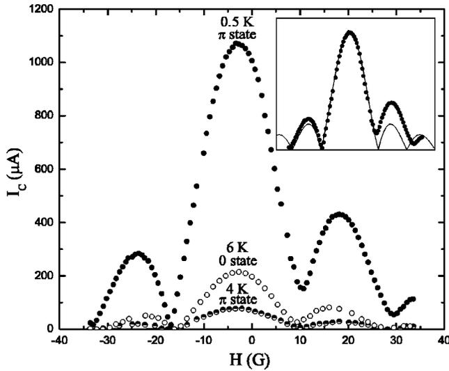
FIG. 11. Critical current versus magnetic field for a Nb/Cu<sub>52</sub>Ni<sub>48</sub>/Nb junction with  $d=18$  nm. These curves do not move with temperature and the critical current disappears completely (for all fields) at the crossover temperature of 4.3 K. Inset: comparison with the ideal Fraunhofer diffraction pattern (solid line).
