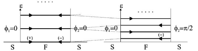
FIG. 2. Discrete spectrum of Andreev bound states in a long one-dimensional ballistic (a) S/N/S junction and (b) S/F/S junction with  $E_{ex} = (\pi/2) E_{Th}$ . Each degenerate state is split by the phase difference  $\phi = \pi/2$  into states carrying currents in opposite directions. The first state above the Fermi level has the largest contribution to the total supercurrent which is positive for the S/N/S junction and negative for the S/F/S junction.
