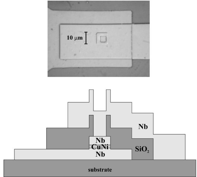
FIG. 8. Photograph and cross section of a device: a square junction of  $10 \times 10 \mu\text{m}^2$  is etched in the Nb/Cu<sub>52</sub>Ni<sub>48</sub>/Nb trilayer and the contact is made on the top through a window in a SiO<sub>2</sub> layer.
