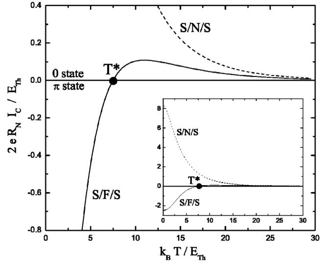
FIG. 5. Crossover between 0 and  $\pi$  states at a temperature  $T^*$  resulting from a nonmonotonic dependence of the critical current in a long S/F/S junction with  $E_{ex} = 13 E_{Th} \ll \Delta$  (solid line), compared to the monotonic behavior of S/N/S junctions (dashed line). The inset shows the same curves on a larger scale.
