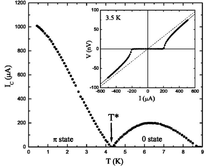
FIG. 10. Critical current versus temperature for a Nb/ $\text{Cu}_{52}\text{Ni}_{48}$ /Nb junction with  $d = 18 \text{ nm}$ . The cancellation at  $T^*$  corresponds to a change of the critical current sign and therefore to a crossover between a 0 state and a  $\pi$  state. Inset: voltage-current characteristic at 3.5 K (the solid line is a fit using the RSJ model and the dashed line represents the normal resistance).
