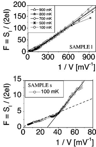
FIG. 5. Fano factor vs the inverse voltage for two different samples. The Thouless energies are  $7 \mu\text{V}$  for sample 1 (top panel) and  $30 \mu\text{V}$  for sample *s* (bottom panel). The solid lines have slopes  $200 \mu\text{V}$  (top) and  $340 \mu\text{V}$  (bottom). In the bottom panel, the incoherent regime is also clearly visible [dashed line is a fit according to Eq. (1)].
