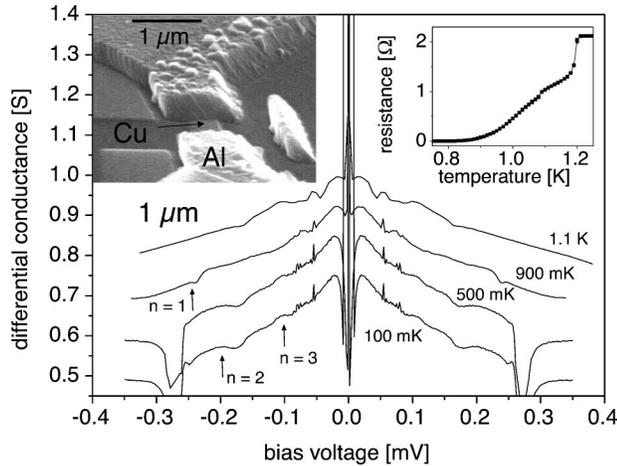
FIG. 1. Differential conductance  $dI/dV$  vs bias voltage at various temperatures for sample 1 (data are shifted by 0.1, 0.2, and 0.35 S for  $T=500$  mK, 900 mK, and 1.1 K, respectively). Left inset: scanning electron micrograph of a typical sample. Right inset: resistance of the sample as a function of temperature. The drop at  $T=1.2$  K is due to the superconducting transition of the aluminum reservoirs.
