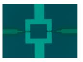
SQUID geometry with two Al-Ge-Al superconducting transistors in a loop.
